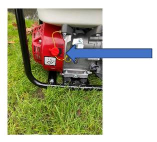
Turn Fuel to ON Push Choke to Left Open Speed lever to half Then Pull Cord to start engine on pump. Push Choke to right until engine runs smoothly
