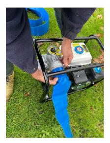
Connect the blue pipe (numbered on pipe end) to get the desired length.
